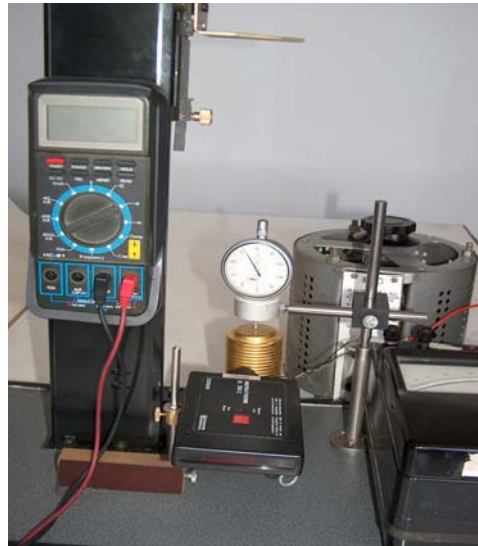
Figure 2. Experimental stand for testing the paraffin electromechanical actuators.
